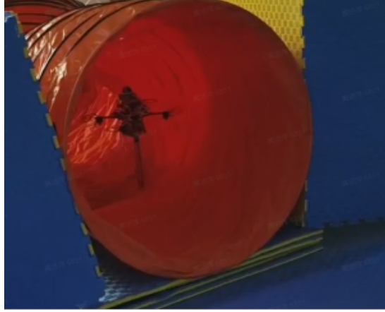
图 3: The quadrotor fixed inside the PVC CANVAS narrow flight tunnel.
